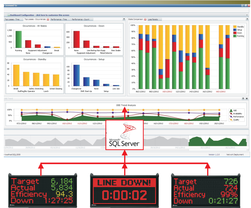
Analyze Complex Production Data - This Production Tracking chart showcases the automated data from multiple Vorne XL units.
